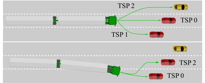
Fig. 6: Illustration of the actuation requests and the corresponding TSP in a lane change to right lane manoeuvre. In the first part of the manoeuvre, the actuation request connected to the TSP defined for the lane to the right of the truck lane (TSP 1) is used for control (top). When the vehicle has shifted to the target lane, the actuation request connected to the current lane (TSP 0) is used for control (bottom).
