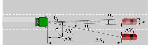
Fig. 2: Illustration of the optical parameters used in the driver model. The parameters are: optical size  $\theta_p$ , angle to a near-point  $\theta_n$ , and a far-point  $\theta_f$ . The distance  $w$  is the width of the lead vehicle and  $\Delta X_n$  and  $\Delta X_f$  are the distances to the near and far-points, respectively.
