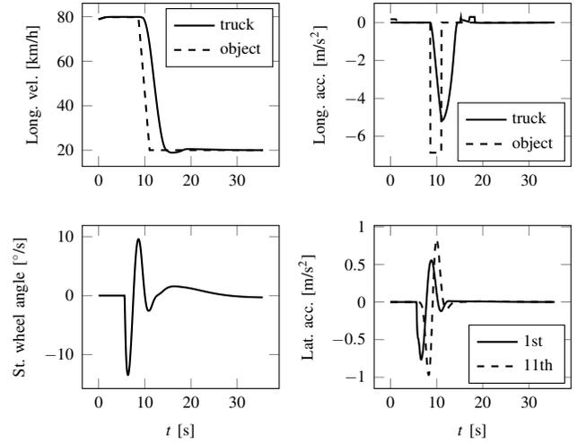
Fig. 11: Important characteristics of a lane change combined with braking where the initial and final velocities are 80 km/h and 20 km/h, respectively: longitudinal velocity (top left), longitudinal acceleration (top right), steering wheel angle (bottom left), and lateral acceleration (bottom right). The absolute magnitude of the initial headway to all vehicles is 2.2 s and the margin value for lane change initialisation is 2.0 s.
