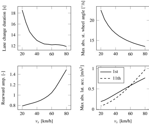
Fig. 10: The main characteristics of lane changes at constant velocities in the range of 20-80 km/h: lane change duration (top left), maximum absolute steering wheel angle amplitude (top right), rearward amplification (bottom left), and maximum absolute lateral acceleration amplitude (bottom right).
