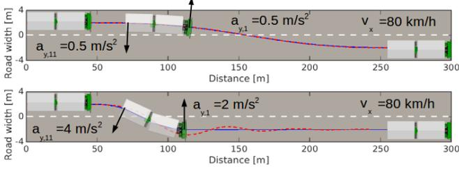
Fig. 1: Illustration of performance characteristics for a LVC in a normal (top) and critical (bottom) highway lane change manoeuvre at 80 km/h with focus on the lateral acceleration rearward amplification and lateral off-tracking. The rearward amplification is approximately 1 in the normal manoeuvre and 2 in the critical manoeuvre. The lateral off-tracking between the first and last axles in the vehicle combination is approximately 0.1 m in the normal manoeuvre and 1 m in the critical manoeuvre.
