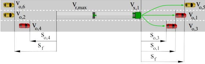
Fig. 4: Closed loop simulations and actuation requests are calculated for the current and adjacent lanes. For each identified lane, the first vehicle ahead and behind the truck within the distance  $s_f$  are identified (red). If no vehicles exists within  $s_f$ , a dummy vehicle (yellow) is defined at  $s_f$ , and given the road speed limit velocity.
