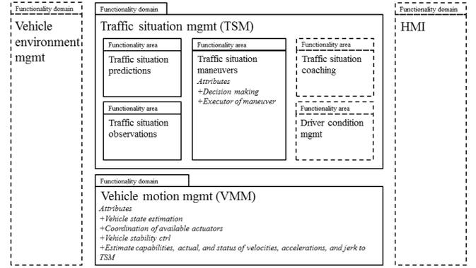
Fig. 5: Function reference architecture: solid boxes are explained, dashed boxes are only for orientation.
