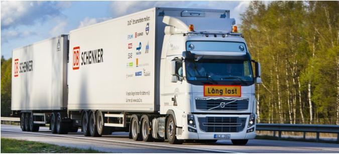
Fig. 1: An example of a LVC. The illustrated vehicle is referred to as an A-double combination.
