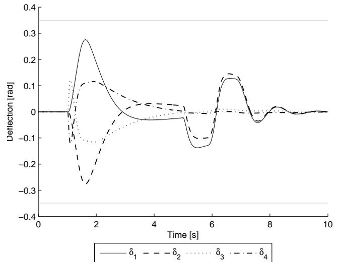
Fig. 10. QP Actuator Response
