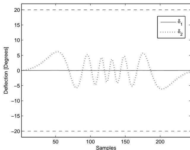
Fig. 3. QP CA Actuator Response
