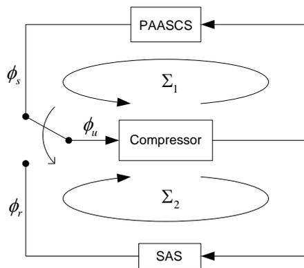
FIGURE 10. Control loop of PAASCS with SAS as the back-up .
