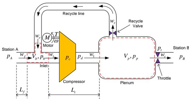
**FIGURE 6.** Compression system with recycle line.
