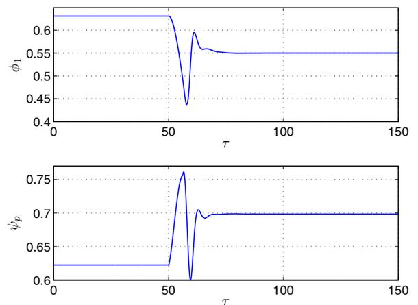
FIGURE 13. Compressor mass flow and plenum pressure of compressor equipped with PAASC and SAS as the back-up when the PAASC is fail.
