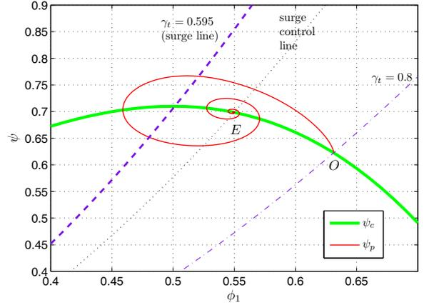
**FIGURE 7.** Close loop trajectory of compressor equipped with SAS during surge.
