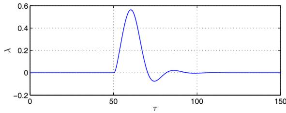
**FIGURE 5.** Piston displacement during the surge stabilization.
