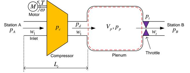
**FIGURE 1.** Model of basic compression system.
