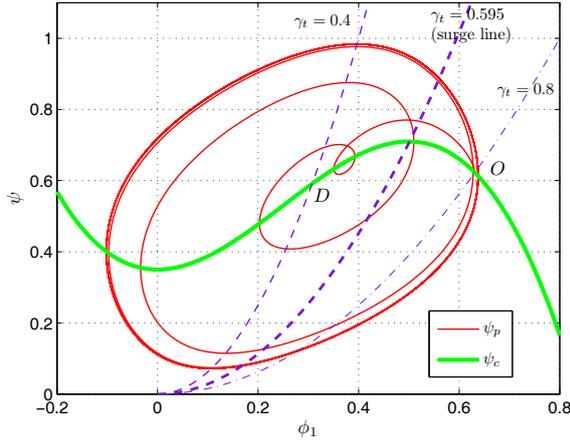
FIGURE 2. System trajectory during surge.
