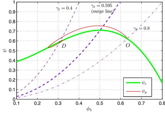
**FIGURE 4.** Close loop trajectory of compressor equipped with PAASCS during surge.
