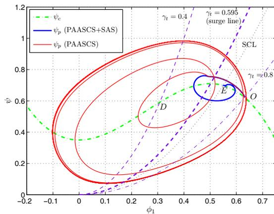
FIGURE 11. Close loop trajectory of compressor equipped with PAASC and SAS as the back-up when the PAASC is fail.
