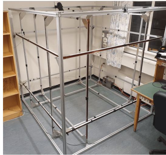
Fig. 3 Assembled Helmholtz cage with two coils per axis.
