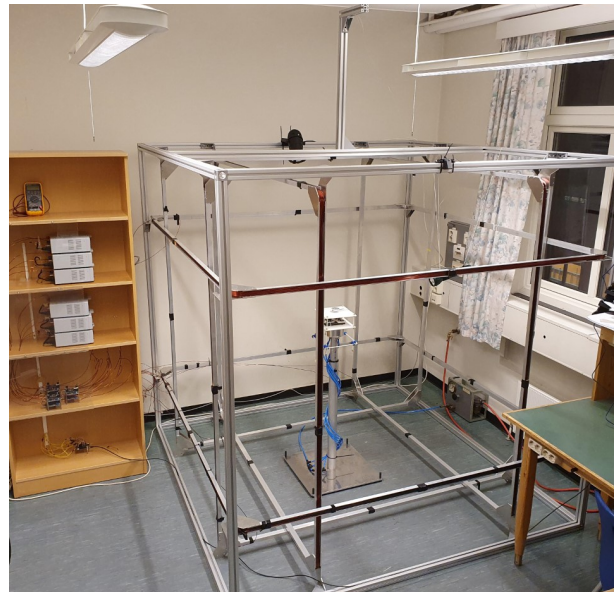
Fig. 7 Complete ADCS testbed with the test-platform balancing, but safely secured, on top of the air bearing.
