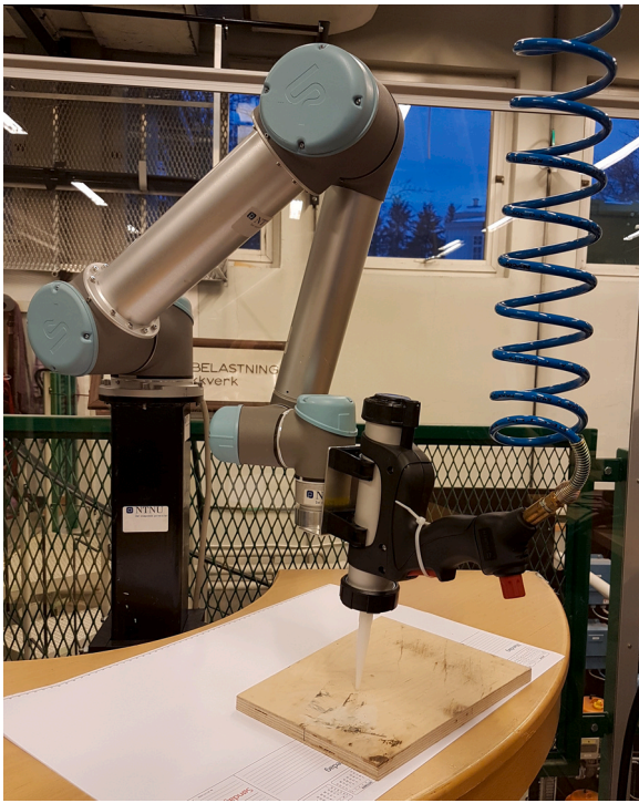
Fig. 1. Robot cell used in preliminary experiments presented in Preliminary tests with viscous material: 6 DOF UR-5 robot manipulator with air-pressure driven caulking gun.
