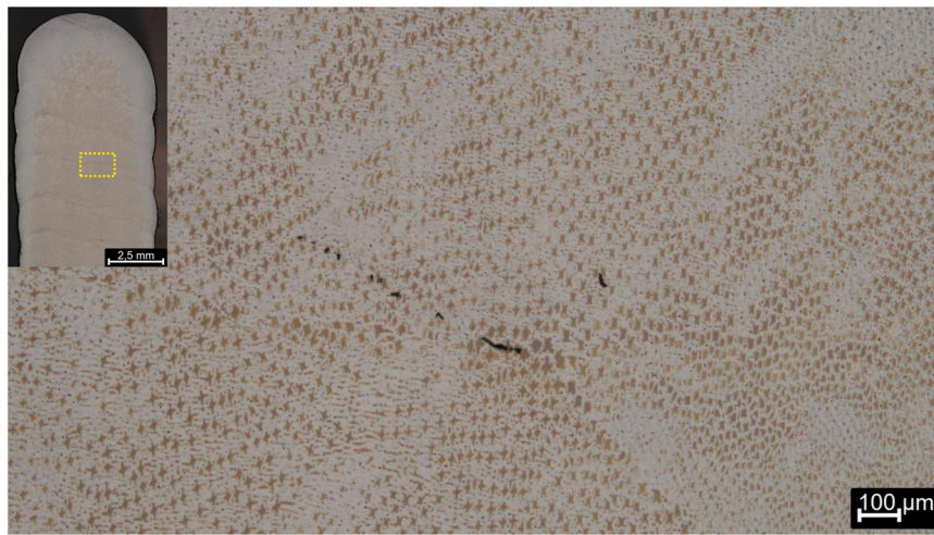
(b) Hexagon corner position with overhang. Structure with fine equiaxed dendrites.
