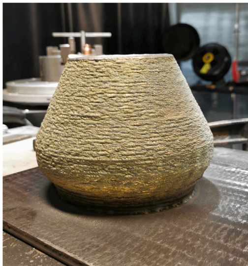
(b) Vase structure, built in UTP 759.
