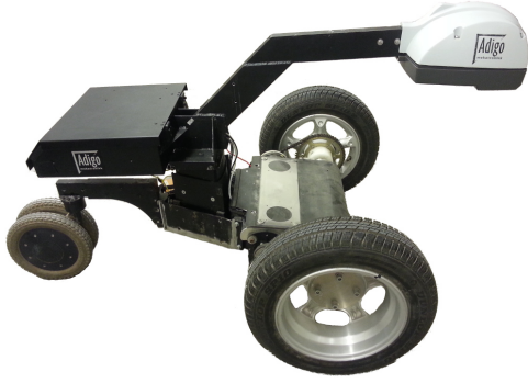
Fig. 4. A picture of the robot used for the tests. The robot uses a rear caster wheel.
