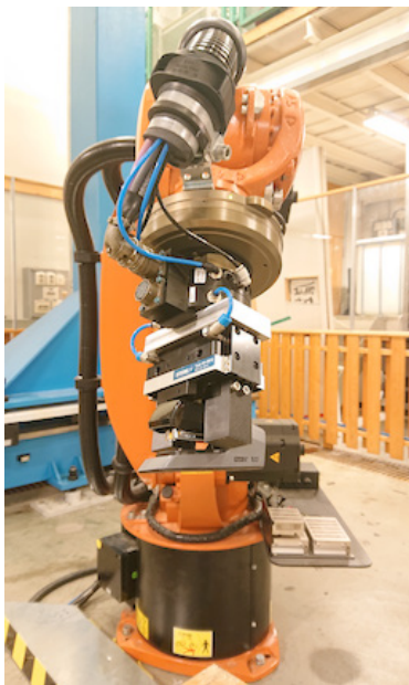
Fig. 9. KR16 ready to transfer the stapler.
