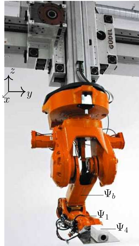
Figure 4.6: The ABB IRB-2400 robot mounted on a GÜDEL gantry crane. The first 5 joints (the 3 of the gantry crane and the first 2 of the robot) are used to generate the ship motion, represented by \Psi_b , and the last four joints of the robot, represented by \Psi_{1,2,3,4} , are used for optimal motion planning of a 4-DoF robot. Links 2 and 3 of the robot are hidden in the wrist and cannot be seen in the figure. Courtesy ABB Strategic R&D for Oil, Gas and Petrochemicals.
