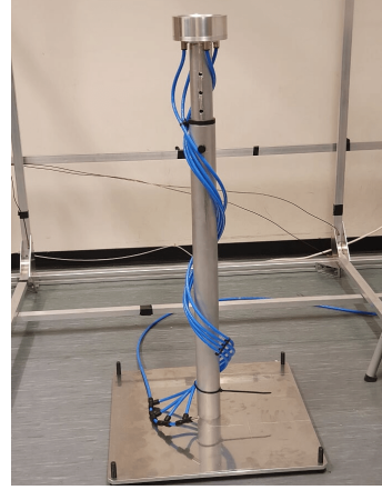
Fig. 4. Image of the completed test stand and air bearing.
