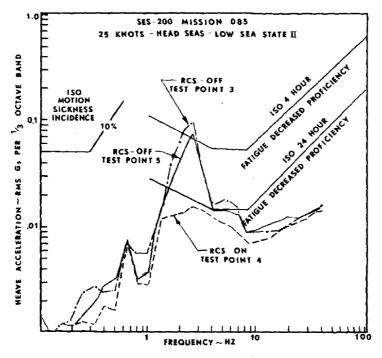
Figure 1.17: Heave accelerations for SES-200 per 1/3 octave band in low sea state II. Picture taken from [16].
