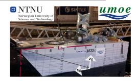
Fig. 3. The picture shows the 3 meter long model test craft of the UM Wave Craft
