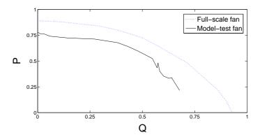
Figure 1.27: Lift Fan Characteristics. The actual full-sized, optimal speed, Wave Craft fan are intentionally designed with a safety margin in terms of air flow capacity.
