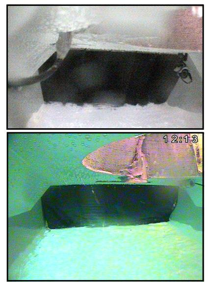
Figure 1.23: Bow and stern seal - seen from the air cushion.
