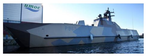
Figure 1.14: The Skjold class, maximum speed of 60 knots+ and overall extreme performance, by courtesy of UM.
