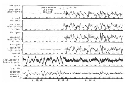
Figure 1.16: RCS turned ON at 14:39:15. Head sea, 3ft waves, 100-ton craft (SES-100A or SES-100B) in 35 knots. Picture taken from [26].
