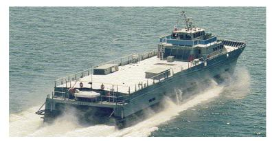
Figure 1.12: The SES 200 had a range of 3000 miles at 25-30 knots without having to refuel.
