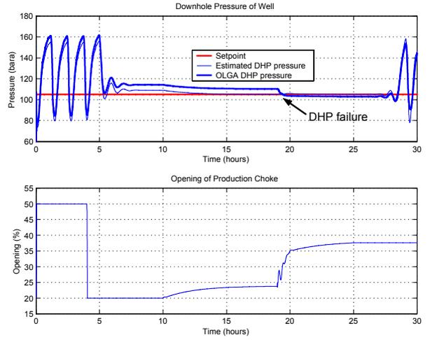
Fig. 5. The estimated and the OLGA downhole pressure for the well. The OLGA well is stabilized by stabilizing the estimated downhole pressure.
